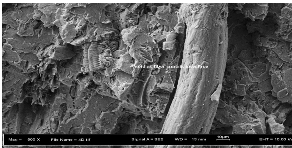
Figure 8 SEM micrograph of the fractured surface of the PVC composite filled with ungrafted OPEFB. A void is shown at the fiber-matrix interface.
